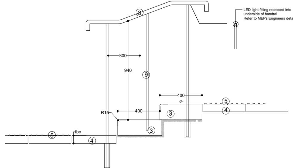
**Typical Section B-b: Typical step**
